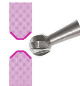
STEP 2: SUPERFICIAL MILLING OF LARGER DIAMETER
